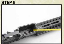
Use airsoft safe silicone to lubricate the hop up chamber. Use sparingly.
