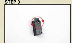
Adjust the velocity screw with a 3/32" allen
