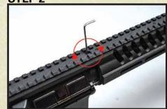
To increase the hop up setting, rotate the hop up dial with a 7/64" allen (Clockwise) towards hop.
