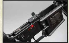
Remove upper manifold by pushing the small pin
