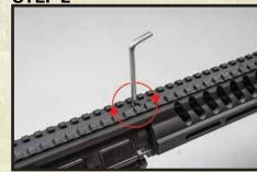
Turn off the hop up by turning the large hop up screw with a 3/16" allen clockwise
