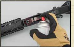
Use airsoft safe silicone to lubricate the hop up chamber. Use sparingly.
