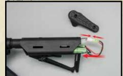
Connect the battery leads. Insert the battery into the stock.
