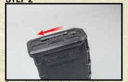
Rotate the wheel on the bottom of the magazine until you hear the clicking sound change.
