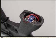
Please check the motor wiring connections.
