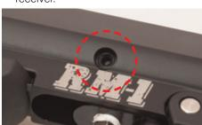
6. To increase or decrease the velocity of the paintballs discharged from a marker, use a 5/32" allen wrench to turn the screw clockwise to reduce velocity and counterclockwise to increase velocity. Note: When adjusting the velocity, make small adjustments, testing after each
